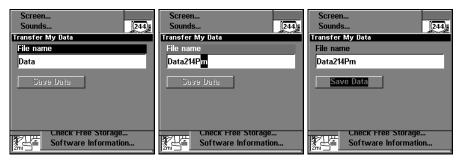
From left to right, these figures show the menu sequence for naming and saving a GPS Data File from the unit's memory to an MMC.
